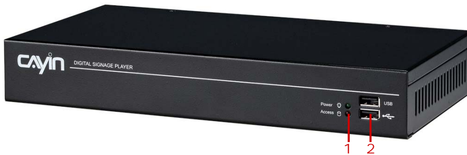
1. Power & HDD LED 2. Front USB connectors
