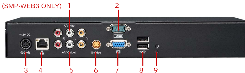
1. AV-in (SMP-WEB3 ONLY) 2. COM Port 3. Power Connector 4. Ethernet 5. AV-out 6. S-Video Out 7. VGA Connector (Output) 8. USB Connectors 9. Power Switch
